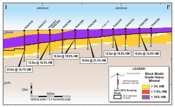
Figure 4: Cross section looking NW through up-dip part of Thunderbird deposit with infill drilling results
