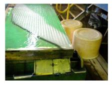
Figure 1: Wet table testwork on bulk samples from left: Yandanooka, West Mine North and McCalls deposits.
