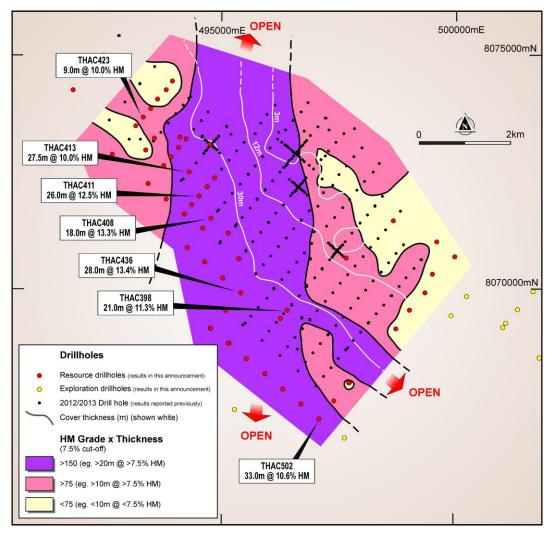
Figure 4: Thunderbird collar plan with HM grade x thickness contours, using a 7.5% HM cut off
