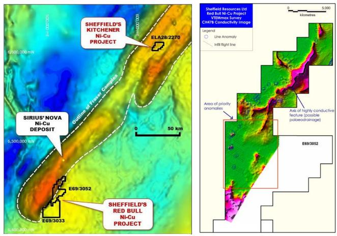
Figure 8: Location of Red Bull Project on a gravity image outlining the Fraser Complex
