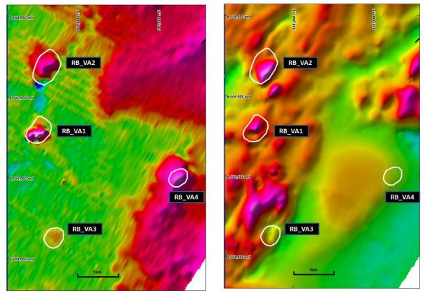
Figures 10 & 11: Late Channel B-field EM (left) and TMI magnetics (right) showing high-order priority targets RB\_VA1 to RB\_VA4. Note the correlating magnetic anomalies for targets RB\_VA1 to 3.
