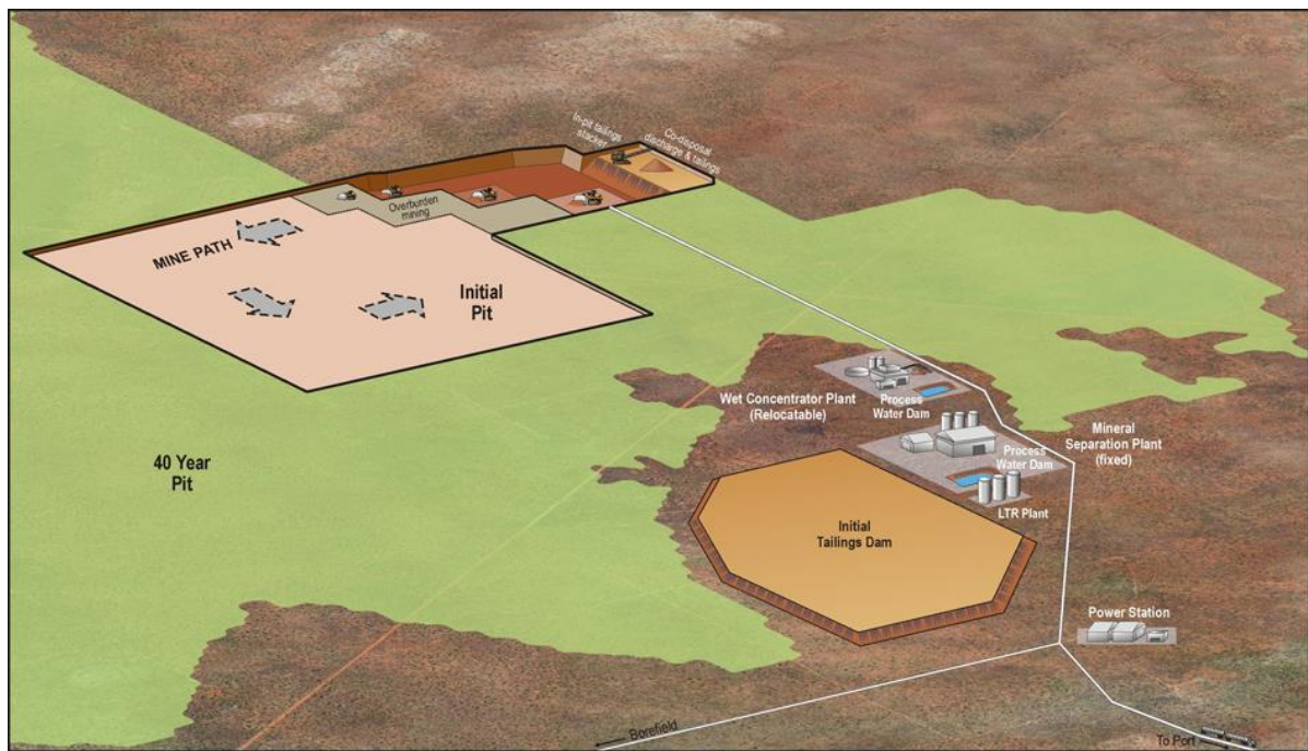
Figure 15: Schematic mine layout with initial pit and 40 year LOM pit shell superimposed (oblique view looking north)
