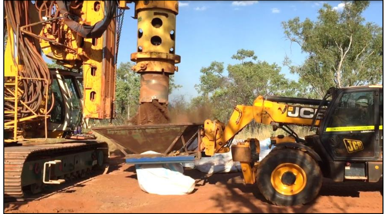
Figure 10: Mineralised Sample Collection from THBA004 using the Bucket Tool (0.7m Diameter)
