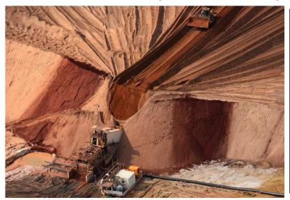
The mining unit plant (MUP) at Thunderbird will reject oversize material (>2mm) via a series of vibrating screens, and will be capable of processing up to 1,500tph.
