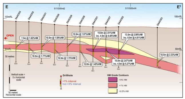
Figure 13: Nomad (2015 aircore drill holes) - Section E-E'
