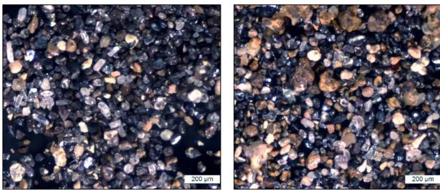
Figure 11: Photomicrograph of HM concentrate from Nomad drill hole DAAC119 (21.0-22.5m) Upper zone (left), DAAC120 (60.0-61.5m) Lower zone (right)
