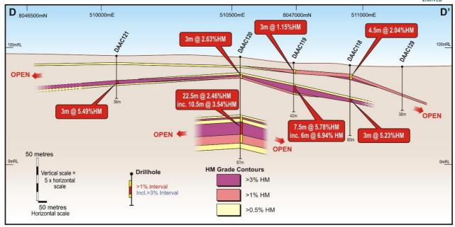
Figure 12: Nomad (2018 aircore drill holes) - Section D-D'
