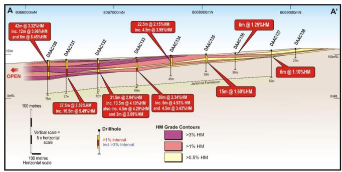
Figure 4: Cold Duck - Section A-A'
