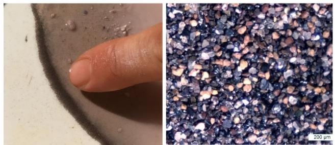
Figure 7: Porphyry Pearl - Panned HM (left), Photomicrograph of HM concentrate drill hole DAAC140 (7.5 – 9.0m)
