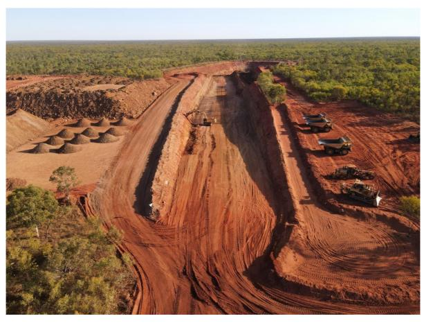
Figure 3: Mine trial pits 1 & 2 and ore and waste stockpiles
