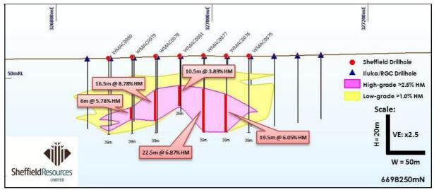
Figure 6: Typical drill hole section through West Mine North (vertical exaggeration x2.5).
