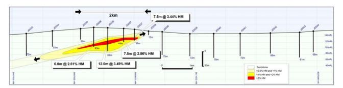
Figure 12: Argo Prospect – Cross Section B-B'
