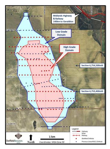
Figure 4: Plan view of the Yandanooka deposit showing holes collars and resource domains
