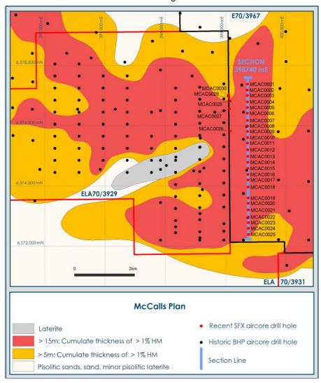
Figure 7: McCalls HMS project – plan of drill hole collars and mineralised zones
