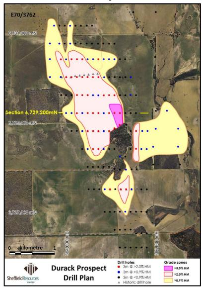
Figure 4: Durack prospect drill plan & mineralised zones
