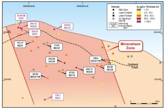
Hill 800 Long section with drill hole intersections projected onto a plane oriented 030 degrees with respect to True North. Note three sub-parallel trends are depicted: Main, Upper Footwall and Lower Footwall, and an interpreted overall trend to the mineralised envelope. In most cases the holes have been drilled oblique to mineralisation, therefore the downhole widths stated may not represent true widths.
