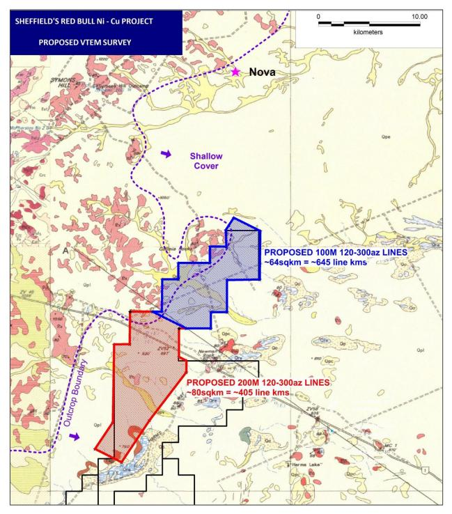
Figure 4: Proposed VTEM survey over GSWA geology relative to Sirius' Nova discovery. GSWA geology map showing the extent of cover (yellow-pale yellow) over Proterozoic basement (pink-red).
