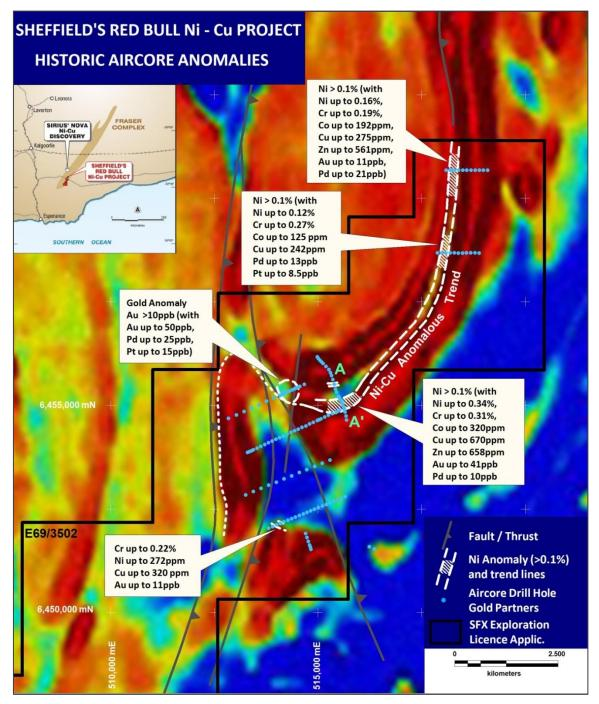
Figure 2: Anomalous aircore drilling results (Gold Partners NL 1995-1997) over TMI magnetic image
