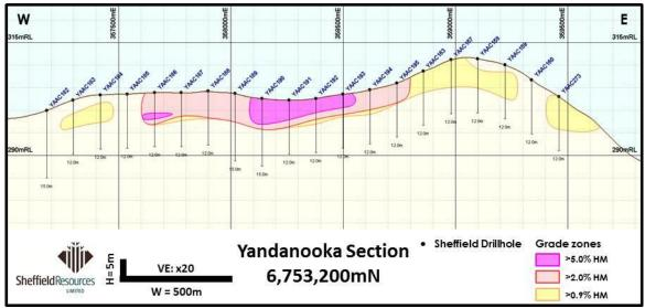
Figure 2: Cross section 7753200mN through the Yandanooka deposit showing the broad mineralised zones and lack of overburden
