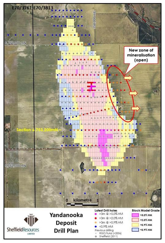
Figure 1: Yandanooka drill hole plan and current resource model. The new drilling either confirms or improves on the predicted model grade.
