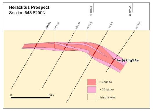
Figure 6: Drill section at Heraclitus prospect showing continuity of anomalous gold mineralisation (Sipa ASX release dated 18 February 2010)
