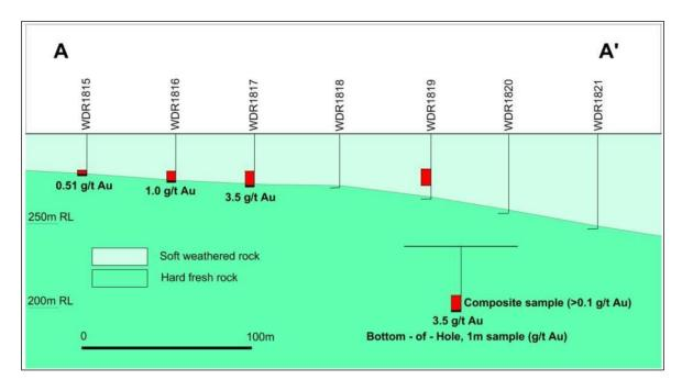
Figure 7: Drill section at Leuccipus prospect with significant gold intersections (Sipa ASX release dated 15 August 2011)
