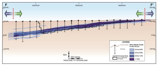
Figure 5: Cross-section F-F' through the Thunderbird resource block model showing the current Resource Zircon grade and April 2014 Scoping Study 32-Year Pit Shell Outline
