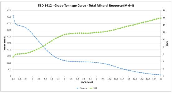
Figure 9: Thunderbird resource grade-tonnage curve.
