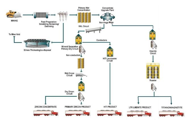
Figure 4: Schematic of Mineral separation Flowsheet - Thunderbird Project
