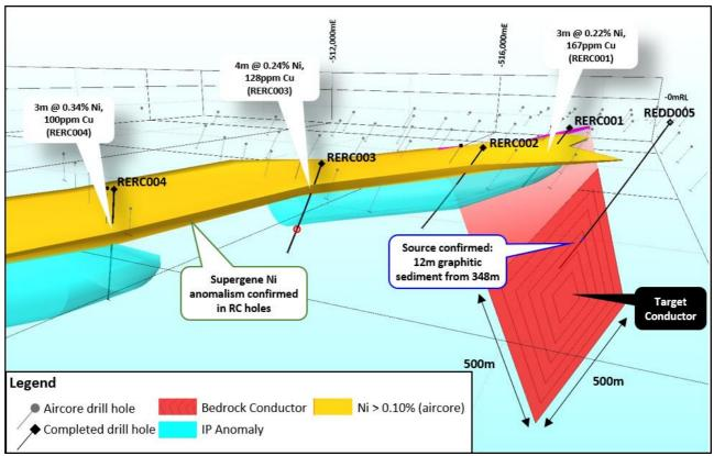
Figure 6: Stud prospect showing drill hole locations and a summary of results
