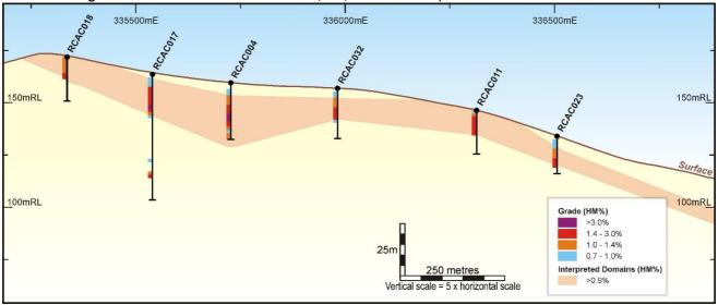
Figure 1.7: Thomson - cross-section 6,696,325mN of interpreted domains and drill holes
