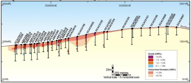
Figure 1.4: Durack - cross-section along 6,729,200mN of interpreted domains and drill holes
