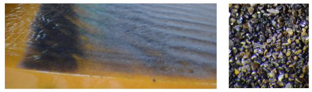
Figure 8: McCalls HM deposit - photo of wet shaking table (left) and photomicrograph of HM (right)
