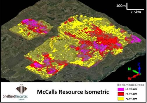
Figure 7: Isometric view of the block model below topography, looking NE
