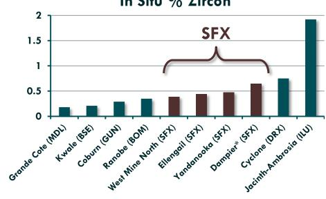
\*The Dampier in situ zircon content is derived by multiplying the weighted average HM content (7.9%) of 8 RIO drill hole intersections by the average zircon content (8%) of the mineral assemblage. RIO's bulk sample metallurgical testwork indicates the zircon content of the HM assemblage could be higher at 11.7%. Refer to ASX release of 7 September 2001 for further details.
