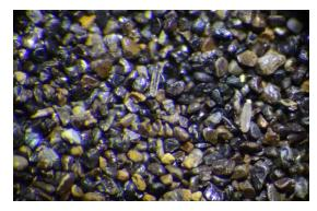
Typical HM concentrate from McCalls: MCAC007 19.5-21m depth, median grainsize diameter 125µm
