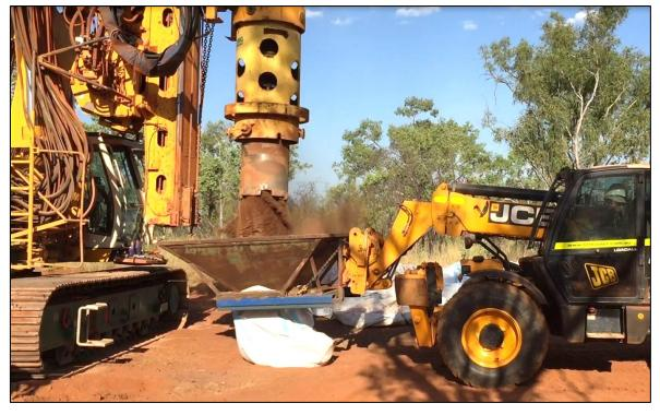
Figure 2: Mineralised sample collection from THBA004 using the bucket tool
