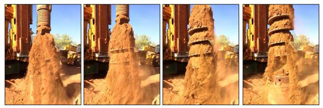
Figure 1: Sequence (from L-R) of mineralisation being lifted from THBA005 using the auger tool (diameter 700mm)
