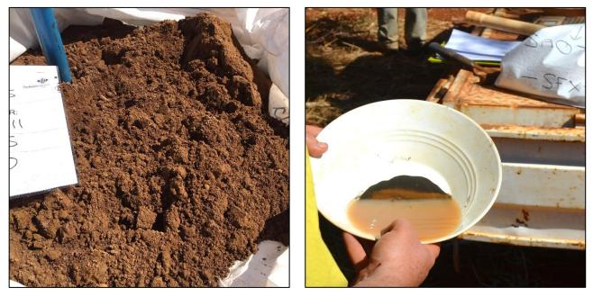
Figure 3: Raw (left) and panned (right) sample – THBA005
