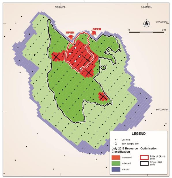
Figure 4: Plan showing location of bulk sample sites and the initial optimised pit shell from the May 2015 PFS
