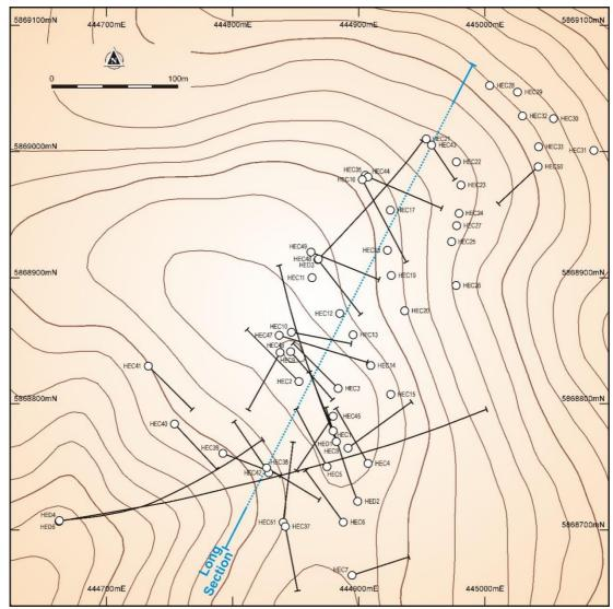
Figure 4: Plan view of historic drilling at Hill 800, with drill traces projected to surface (10m contours).
