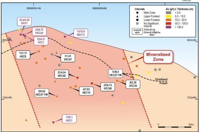
Figure 1: Hill 800 Long section with drill hole intersections projected onto a plane oriented 030 degrees with respect to True North (see Figure 4). Note three sub-parallel trends are depicted: Main, Upper Footwall and Lower Footwall, and an interpreted overall trend to the mineralised envelope. In most cases the holes have been drilled oblique to mineralisation, therefore the downhole widths stated may not represent true widths.
