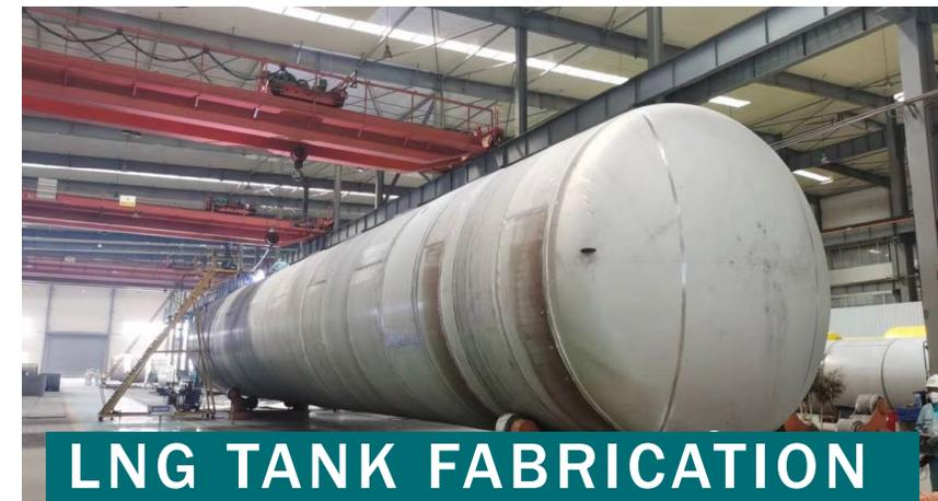
**LNG TANK FABRICATION**
