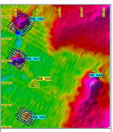
Figure 1: Proposed FLTEM survey arrays over high order VTEM anomalies RB\_VA1-3 (Late Channel B-field VTEM image).
