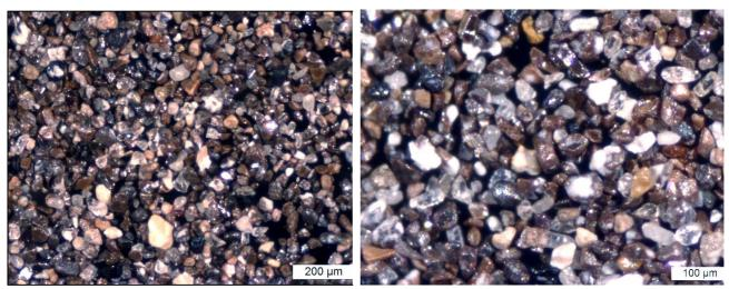
Figure 7: Photomicrograph of HM concentrate from Bohemia, drill hole NLAC017 (19.5-21m)
