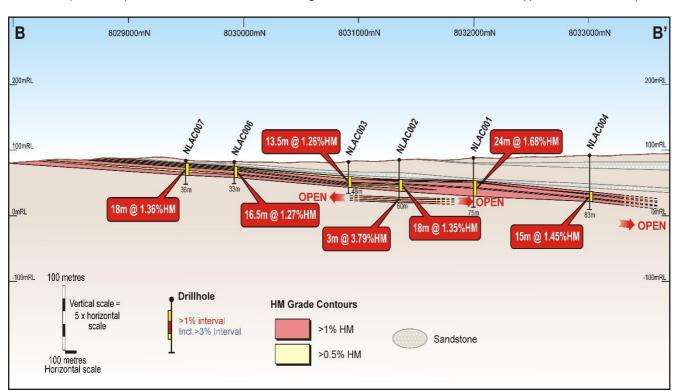
Figure 8: Concorde - Section B-B
