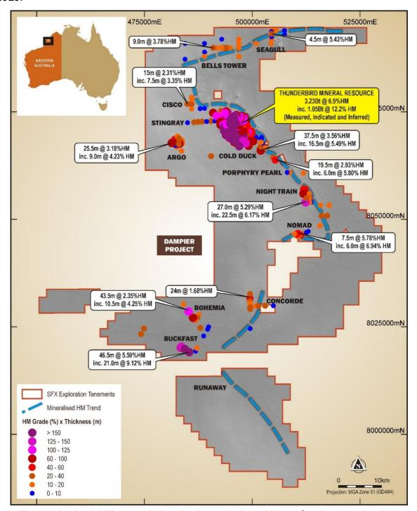
Figure 1: Regional drilling compilation showing grade times thickness<sup>1</sup> and prospect locations
