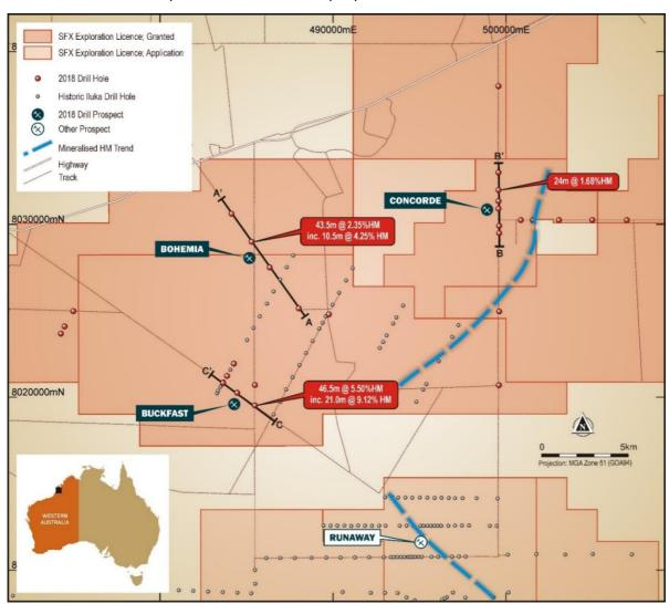
Figure 3: Plan of the Buckfast, Bohemia and Concorde prospects showing significant drill intersections
