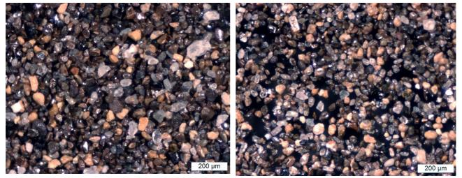
Figure 9: Photomicrograph of HM concentrate from Concorde, left - drill hole NLAC001 (42-43.5m), right - drill hole NLAC007 (12-13.5m)
