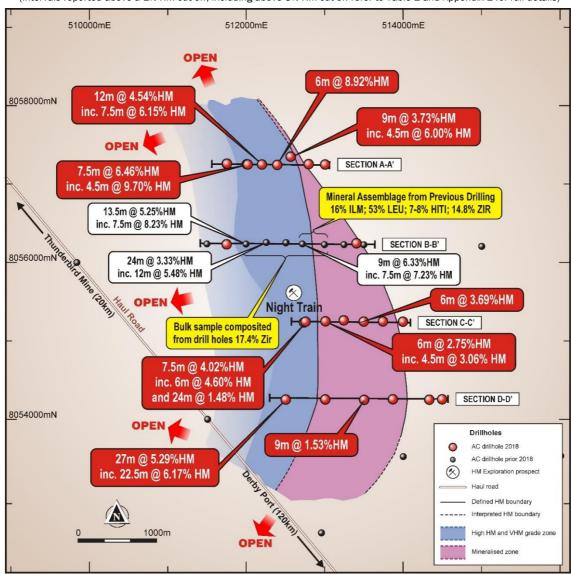
Figure 1: Plan of the Night Train prospect showing significant drill intersections
