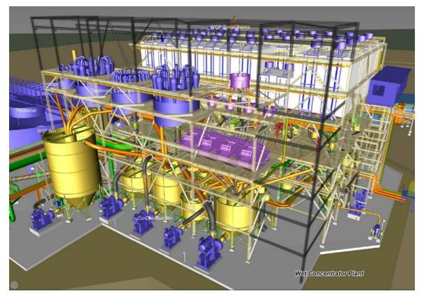
Figure 5: Wet Concentrator design and layout
