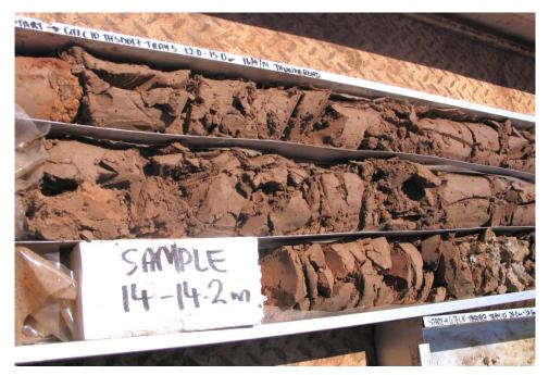
Figure 8: An example of dense sand which constitutes 85-90% of the Thunderbird deposit (the sample has been cut with a hand trowel)
