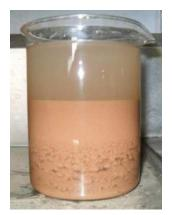
Figure 6: Thickened slimes after 5-10 minutes settling
