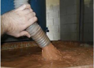
Figure 4: Cyclone overflow (trace +38 micron)
