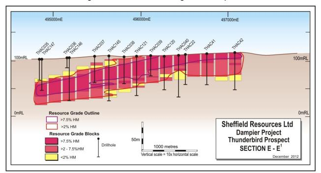
Figure 3: Section E-E' through the Thunderbird resource, showing the change in cover thickness as the dip of mineralisation increases to the south-west
