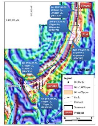
Figure 6: Northern Targets: end-of-hole nickel anomalies from aircore drilling on TMI magnetics
