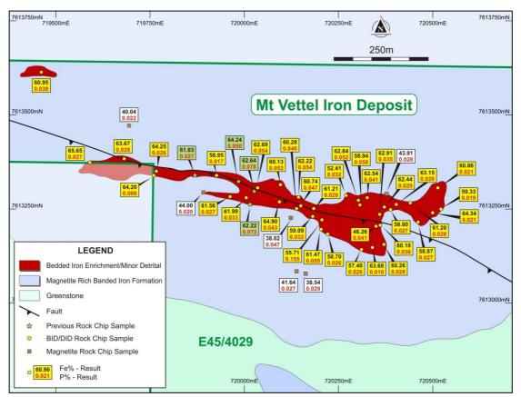
Figure 10: Mt Vettel - mapped iron enrichment and rock chip sample results
