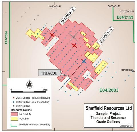
Figure 3: Thunderbird drill collar plan showing location of holes with assay results reported to date, and outline of blocks in the current (Dec 2012) resource above 7.5% HM and 2% HM, projected to surface
