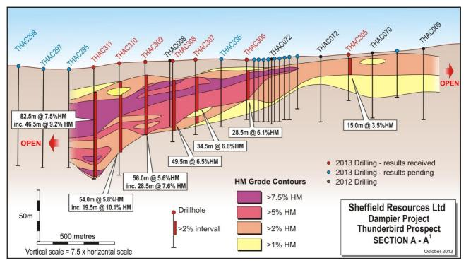
Figure 4: Section A-A', looking northwest showing the excellent continuity between holes of the mineralised envelope (>2% HM), and the higher grade zones (>5% and >7.5% HM)
