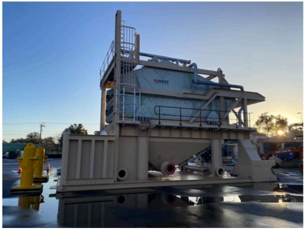
Image 5: Dry Mining Unit Screen Assembly
