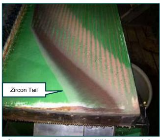
Cleaner stage gravity separation of HM on bulk sample from the Argo prospect. Source: Rio Tinto Exploration Pty Ltd open file report.
