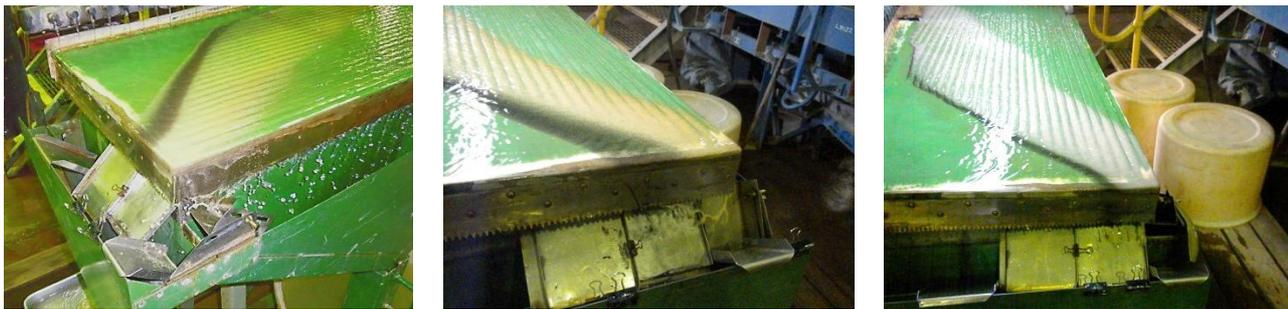
**Figure 1: Wet table testwork on bulk samples from left: Yandanooka, West Mine North and McCalls deposits.**
