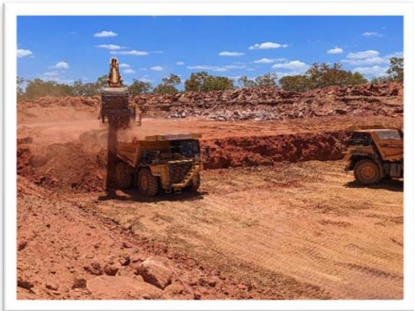
**Figure 2: Waste mining by excavator and truck**
