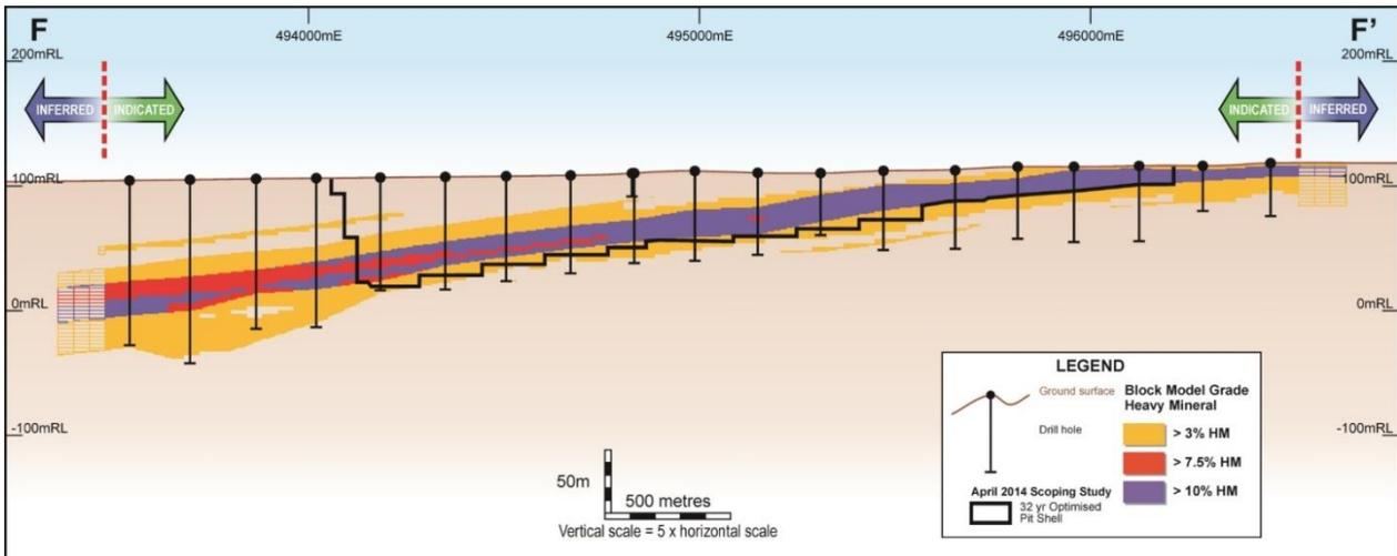
Figure 3: Cross-section F-F' through the Thunderbird resource block model showing the current Resource HM grade and April 2014 Scoping Study 32-Year pit shell outline
