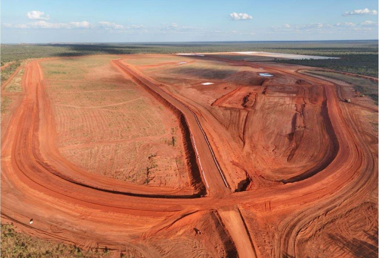
Image 7: Tailings storage facility (foreground) and stormwater storage pond (background)
