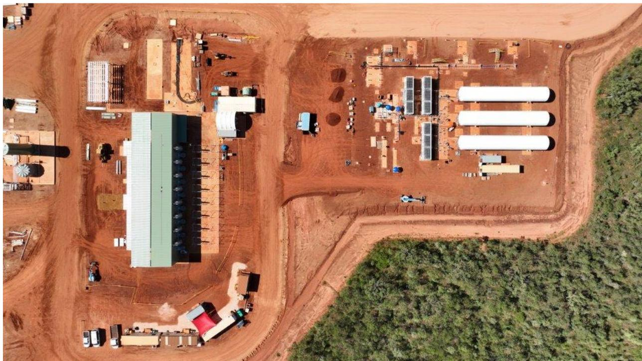
**Figure 5: Power Generation building (LHS) and LNG storage area (RHS)**
