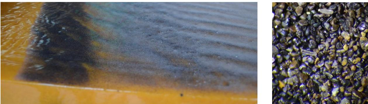
Figure 8: McCall's HM deposit - photo of wet shaking table (left) and photomicrograph of HM (right)
