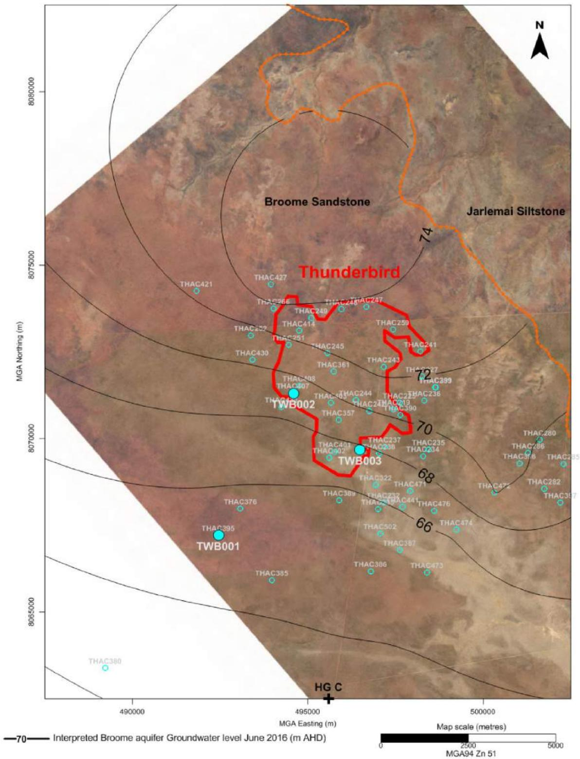
Figure 23: Mine Site Development Envelope Interpreted Groundwater Levels (2016)
