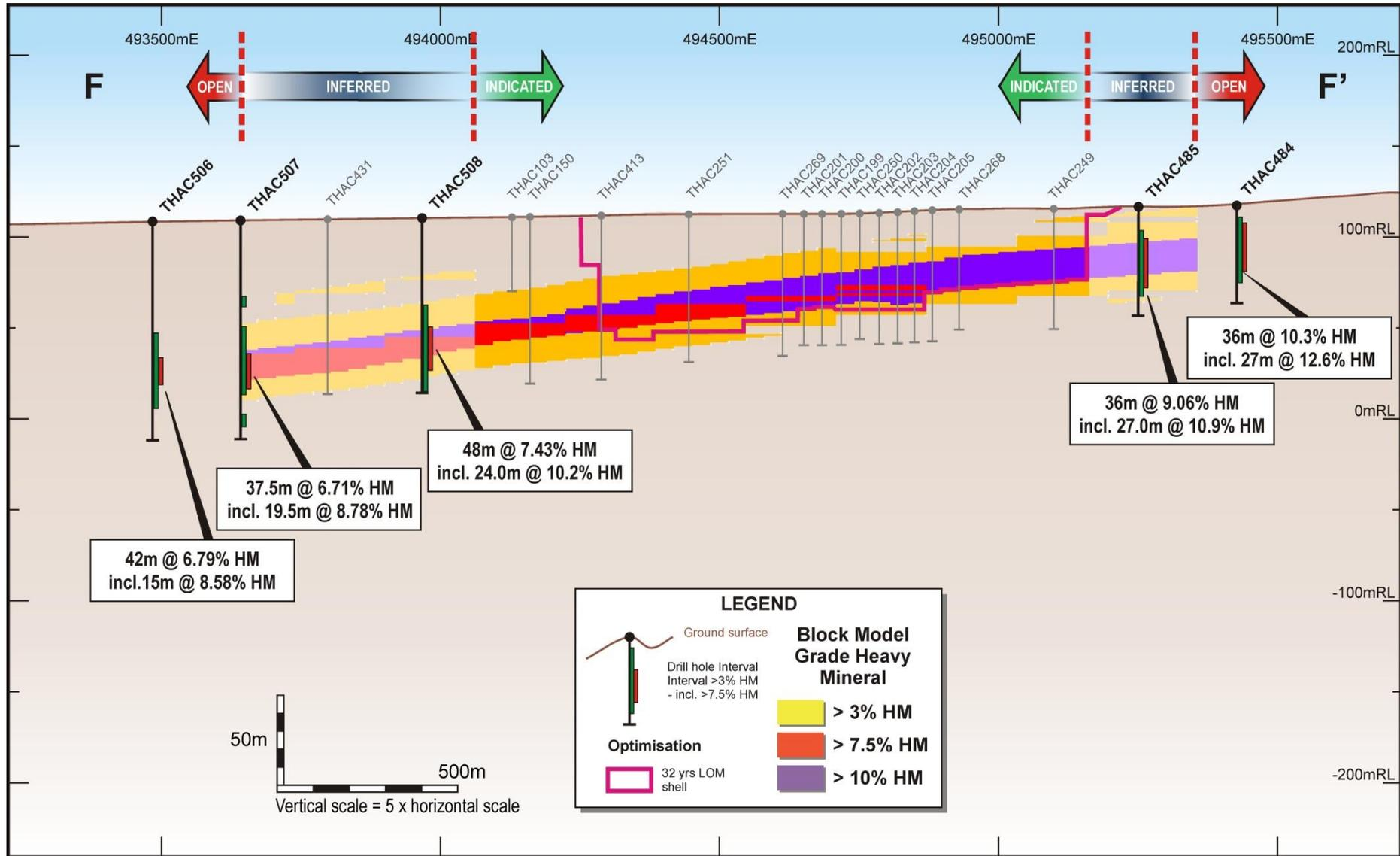
Figure 2: Cross-section F-F' through the Thunderbird deposit showing the resource and 32 year pit shell outline, resource classifications and drill holes in this ASX release.
