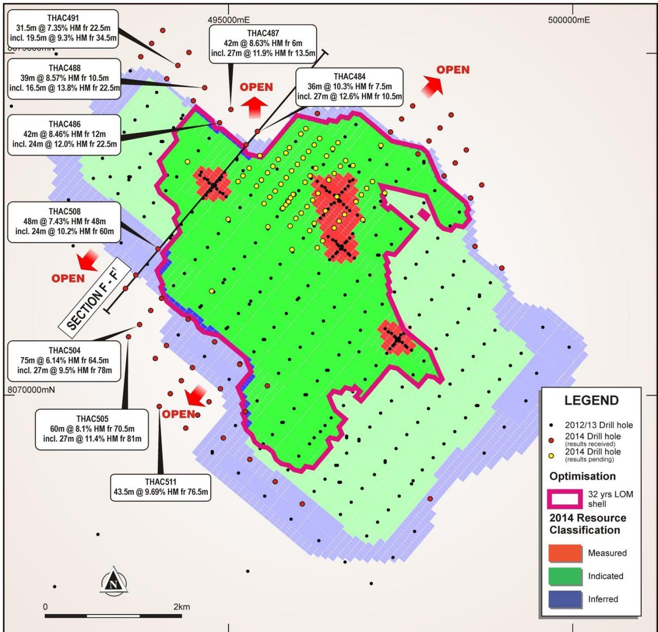
Figure 1: Plan view of Thunderbird Deposit 32-year pit shell outline on Mineral Resource Classifications showing location of drillholes in this ASX release.
