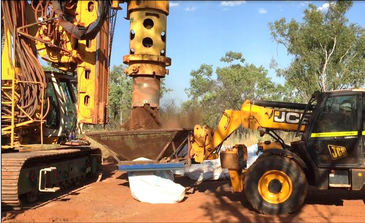
**Figure 2: Mineralised sample collection from THBA004 using the bucket tool**
