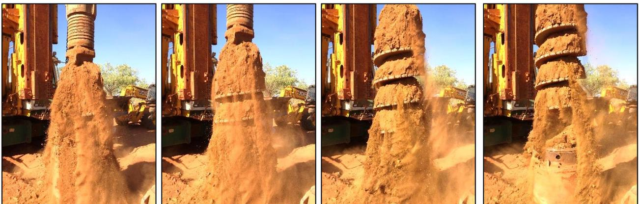
Figure 1: Sequence (from L-R) of mineralisation being lifted from THBA005 using the auger tool (diameter 700mm)
