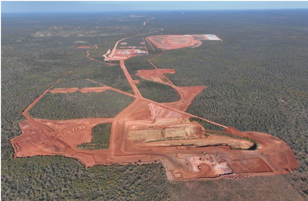
**Figure 7: Thunderbird Mine Site Overview – Mining start-up area (foreground) & Process Plant & Tailings Storage Facility (background)**
