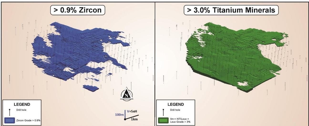
Figure 6: Thunderbird Resource block model >0.9% in-situ zircon left and >3% TiO<sub>2</sub> minerals right
