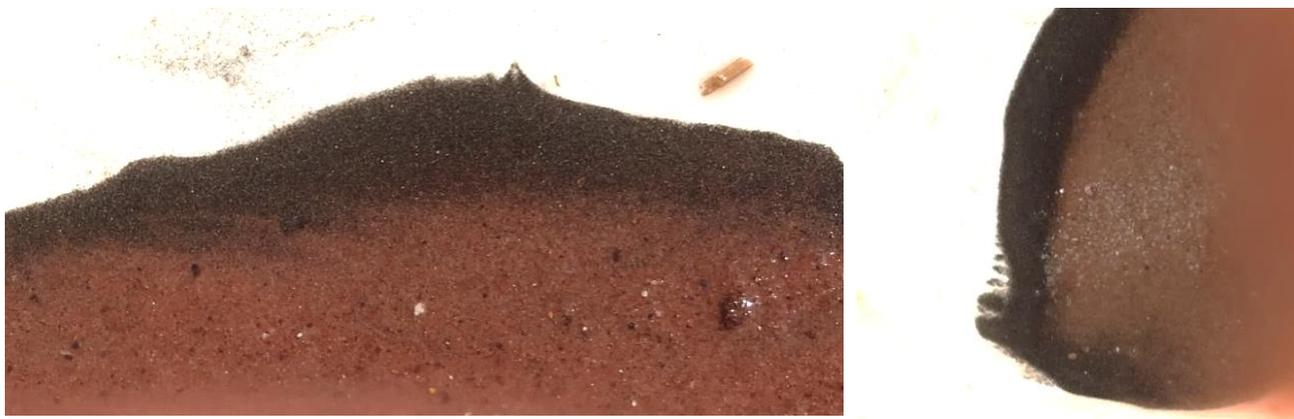
Figure 4: Panned HM hosted by brown sands, from Buckfast drill hole NLAC027
