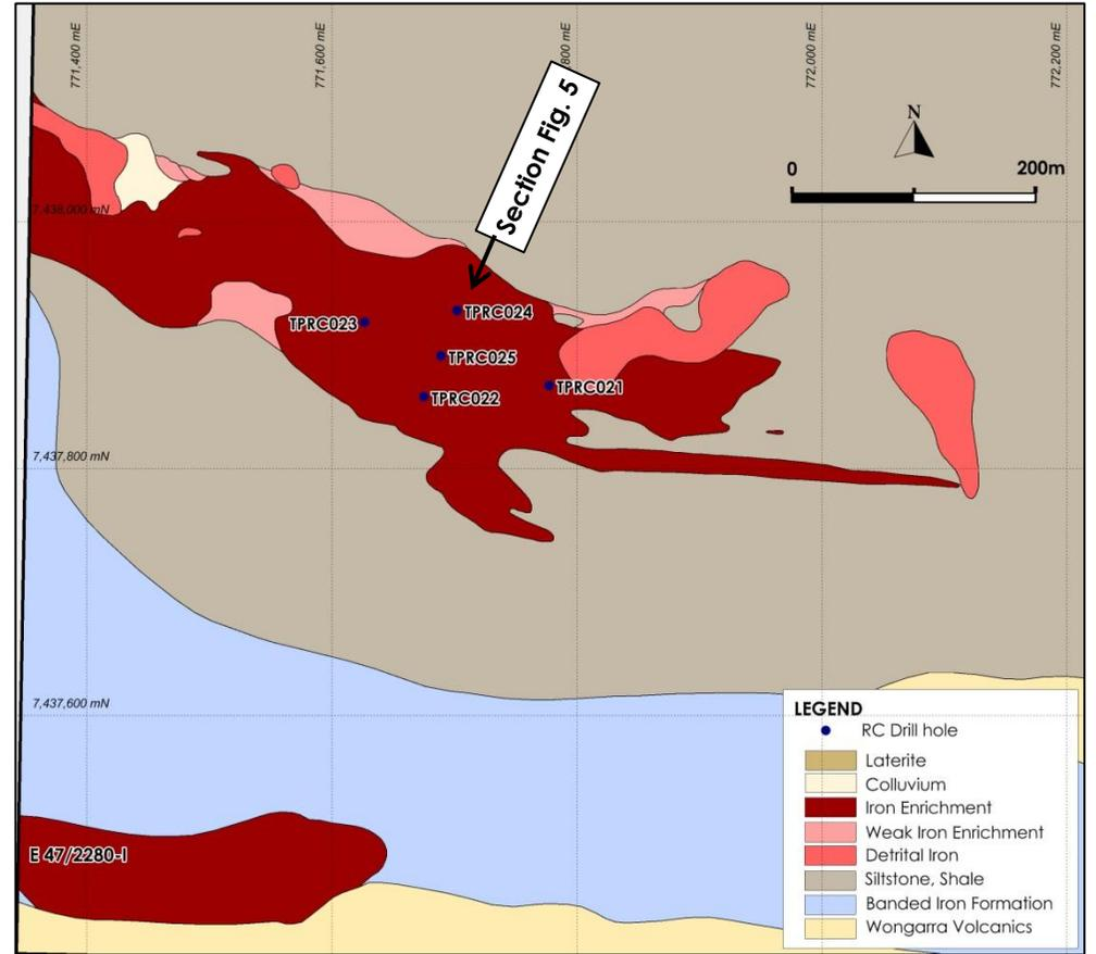
Figure 3: Crucible Prospect surface geology and drill hole locations. Mineralisation mapped at surface remains undrilled to the northwest.
