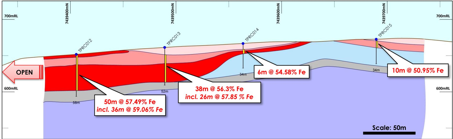
Figure 4: Cross-section through TPRC012 to TPRC015 at the Top Forge prospect.
