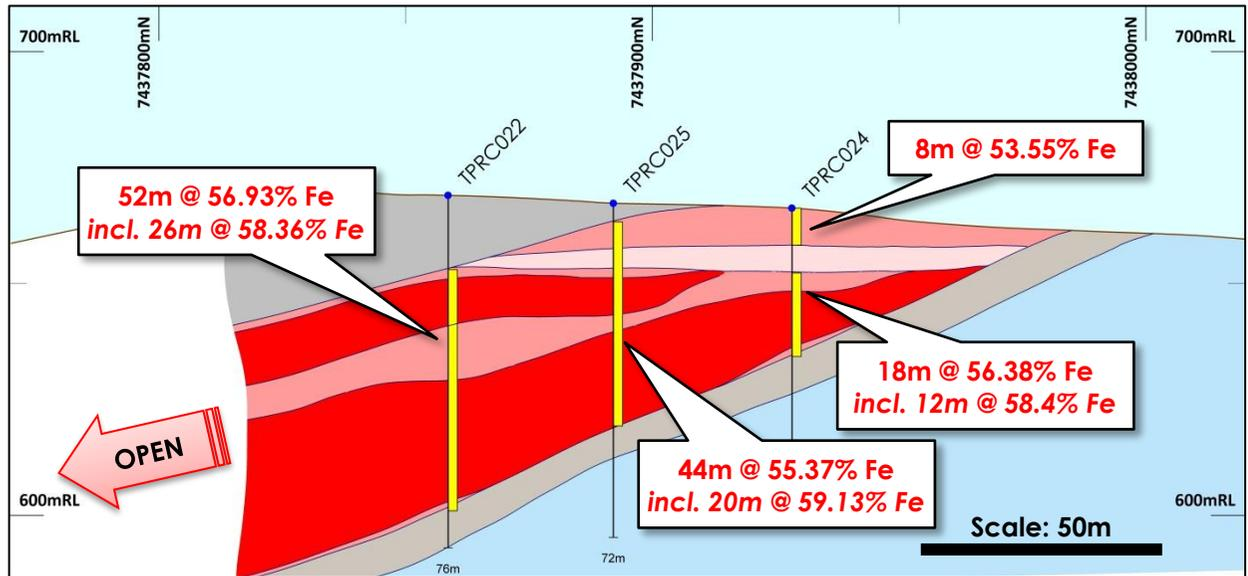
Figure 5: Cross-section through TPRC022, 025 and 024 at the Crucible prospect.
