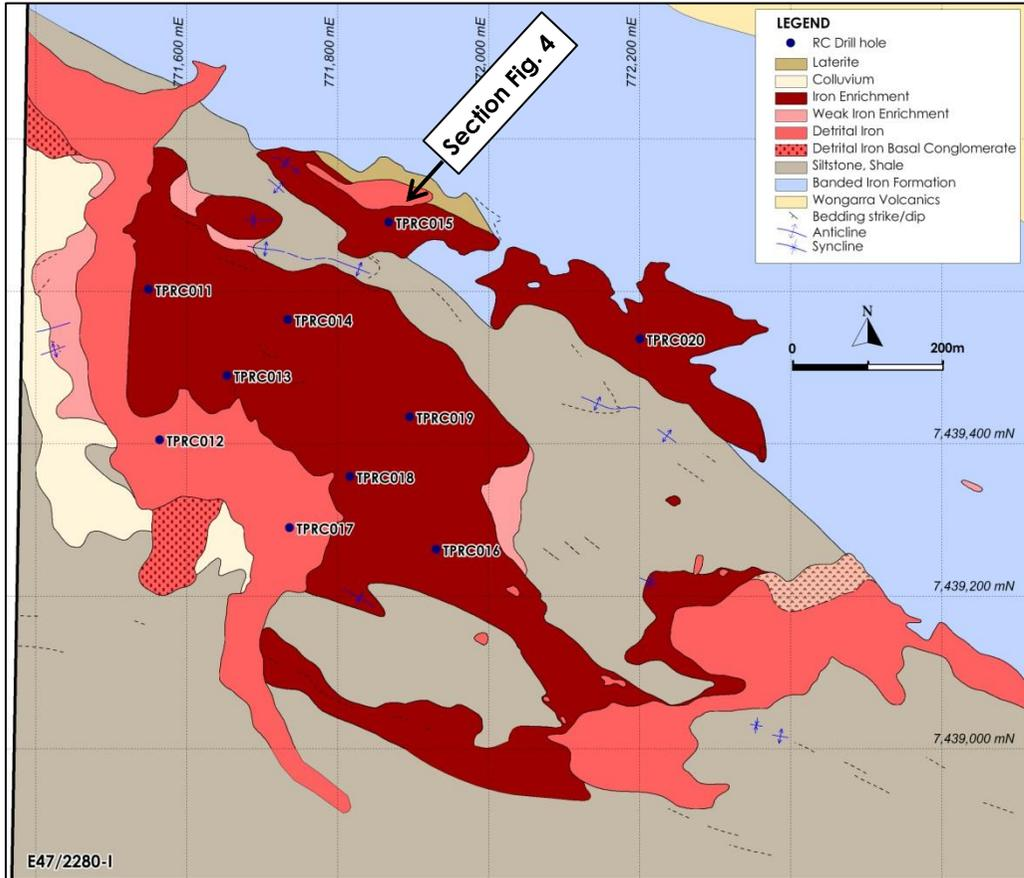
Figure 2: Top Forge Prospect surface geology and drill hole locations. Mineralisation mapped at surface remains undrilled to the southwest and southeast.
