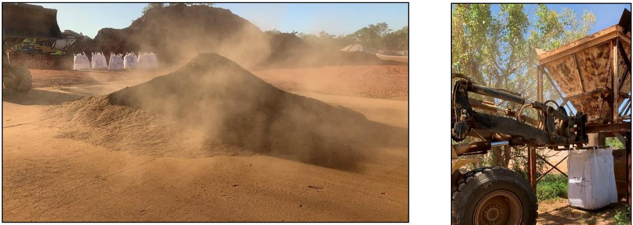
**Figure 2: Homogenisation of bulk sample (left), re-bagging of bulk sample (right)**
