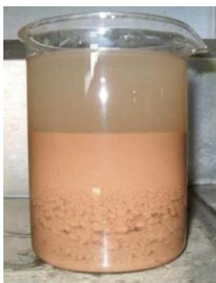
**Figure 6: Thickened slimes after 5-10 minutes settling**
