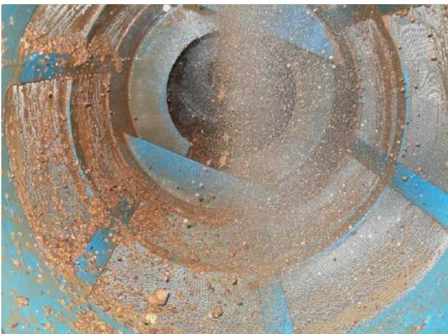
Figure 3: Scrubber/trommel oversize removal
