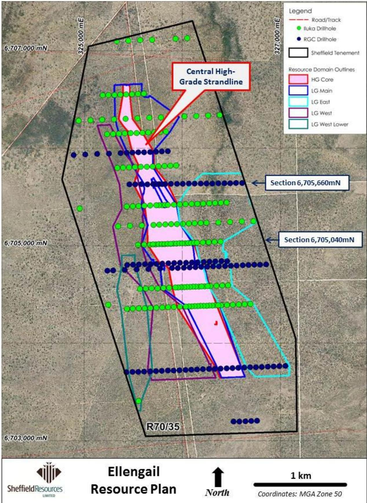
Figure 2: Plan view of the Ellengail Deposit showing holes collars and resource domain outlines
