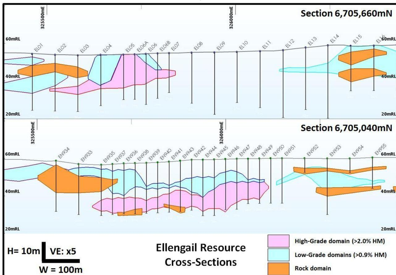
**Figure 3: Typical cross-sections, looking north, through the Ellengail deposit showing resource domain outlines and drill holes.**
