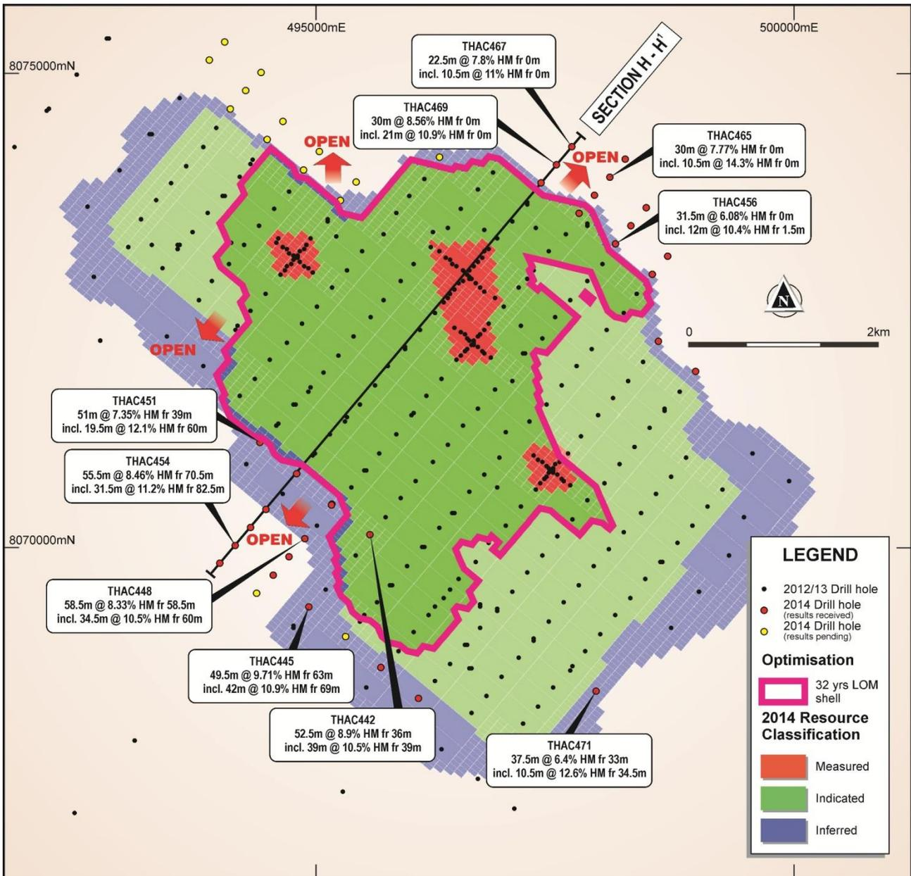
**Figure 2: Plan view of Thunderbird Deposit 32-year pit shell outline on Mineral Resource Classifications showing location of drill holes in this ASX release**
