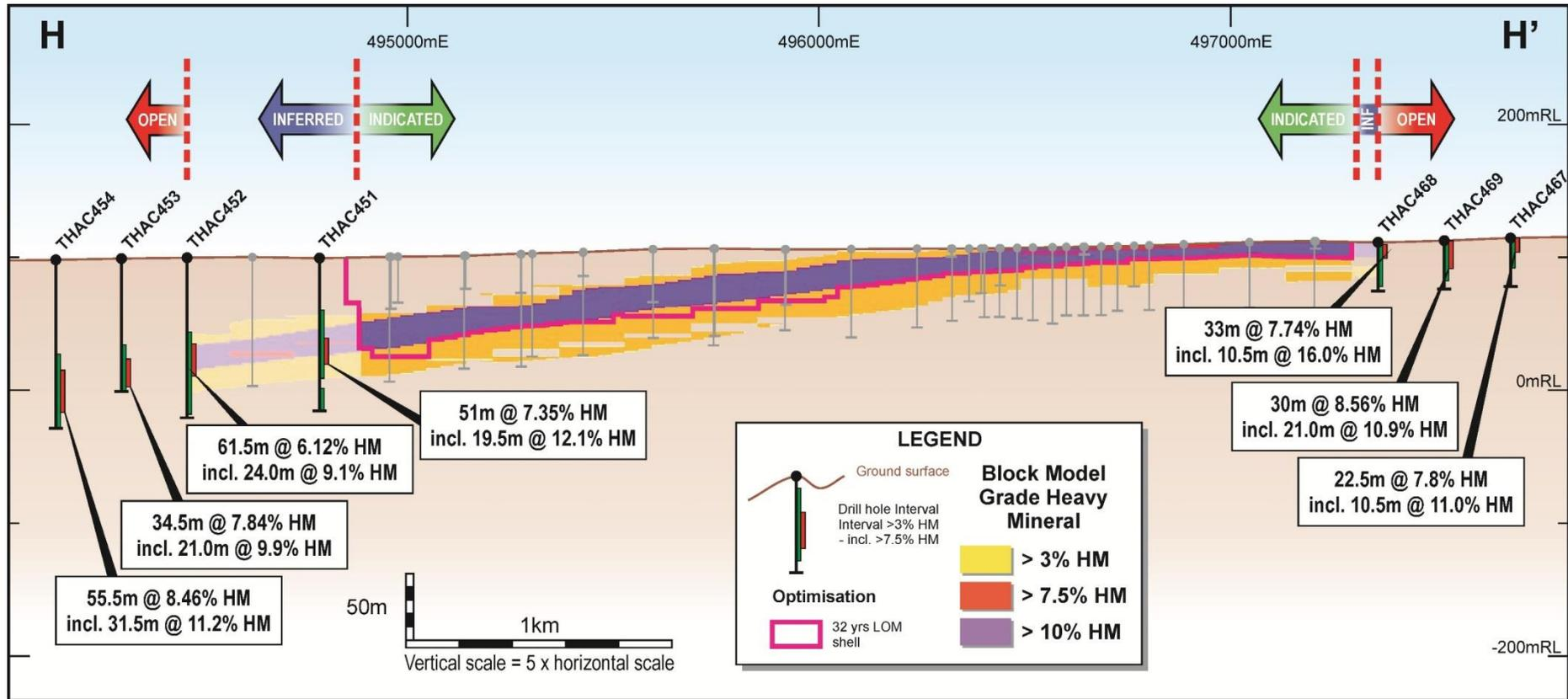
Figure 1: Cross-section H-H' through the Thunderbird deposit showing the resource and 32 year pit shell outline, resource classifications and drill holes in this ASX release
