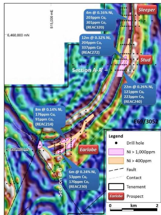
Northern Targets - aircore drilling results
